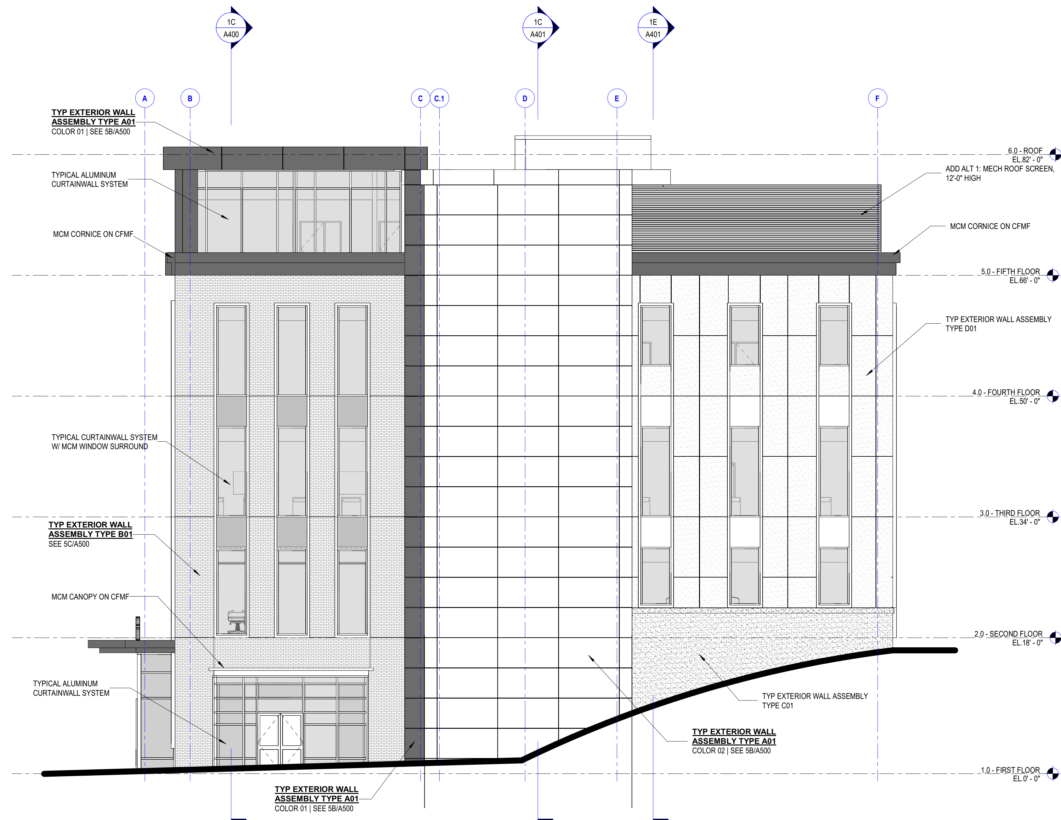
3C BUILDING ELEVATION - WEST 1/8" = 1'-0"
