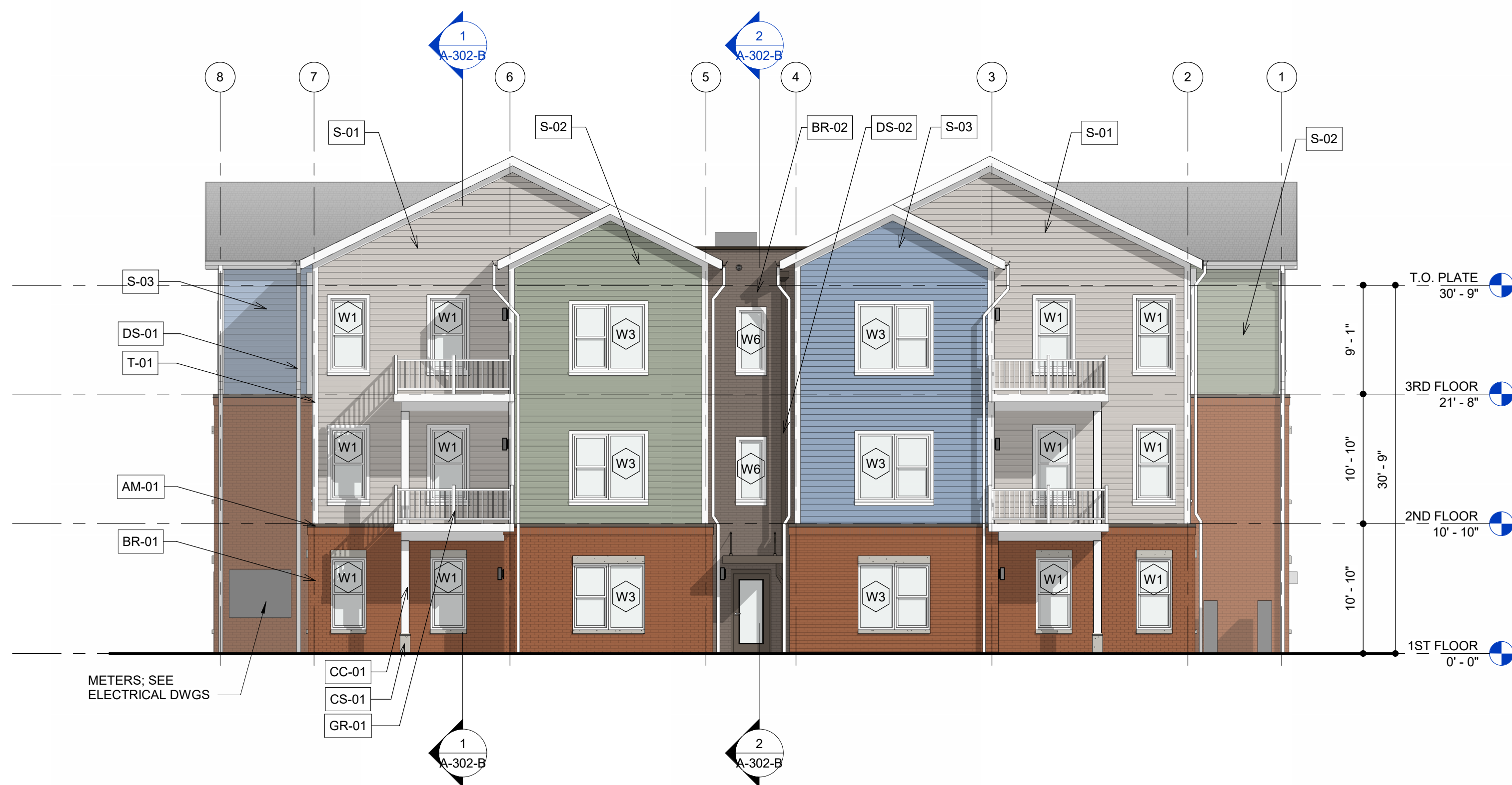
3 BUILDING B NORTH ELEVATION 1/8" = 1'-0"
