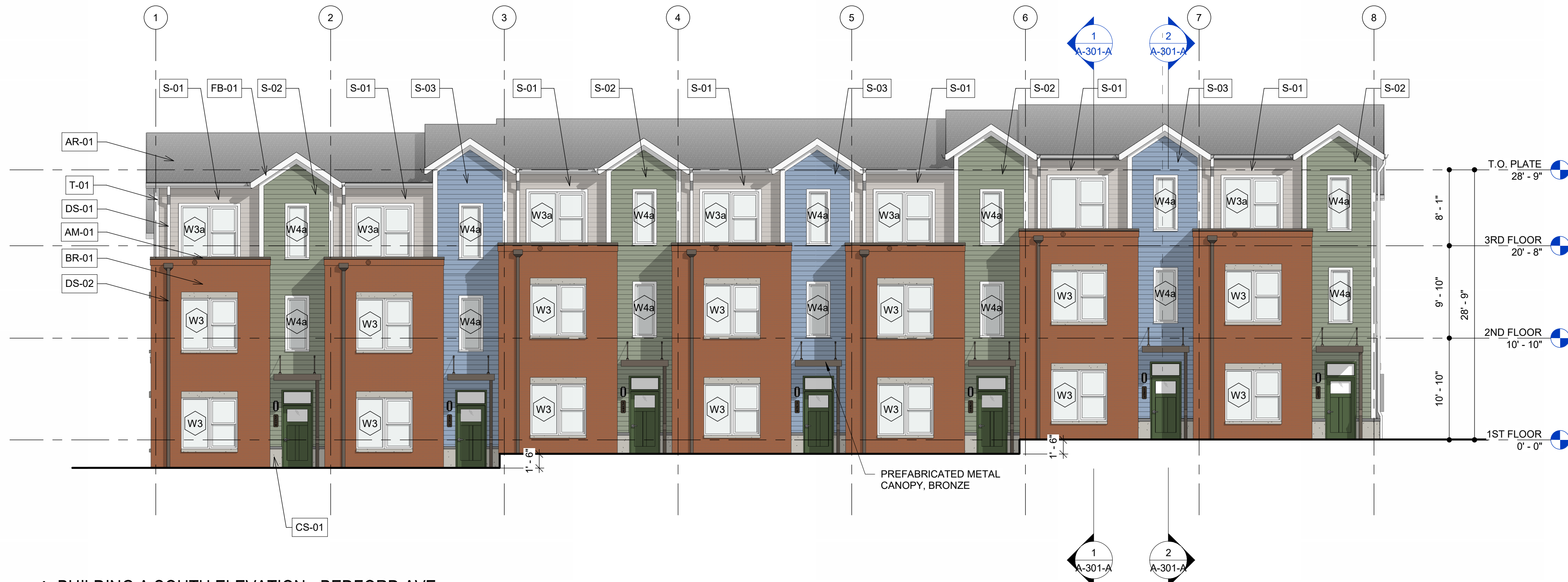
1 BUILDING A SOUTH ELEVATION - BEDFORD AVE 1/8" = 1'-0"
