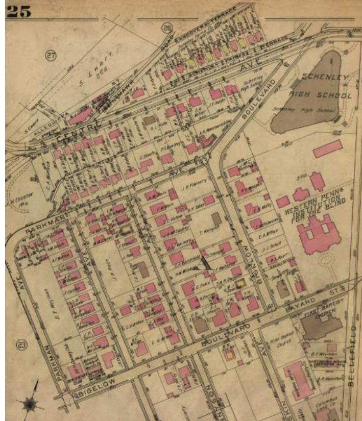
Sanborn Maps can help approximate the date and original materials of a building, and catalogue changes in the area.
